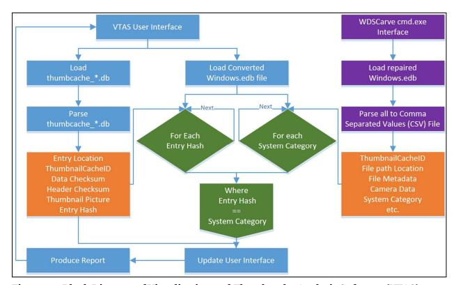
Figure 2 – Block Diagram of Visualisation and Thumbcache Analysis Software (VTAS)
