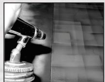
Fig. 11: Airbrushing along the masking.
