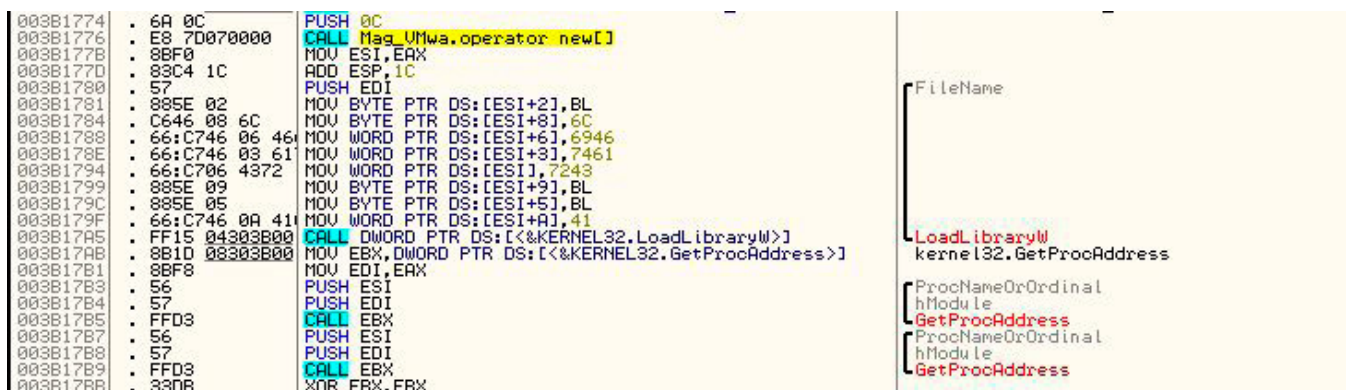
Figure 9. Building CreateFileA as a Character Array
