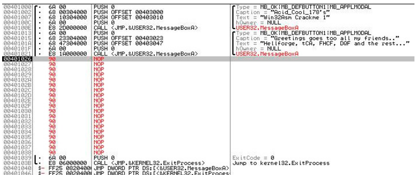
Figure 12. Replaced PUSHes and CALL
