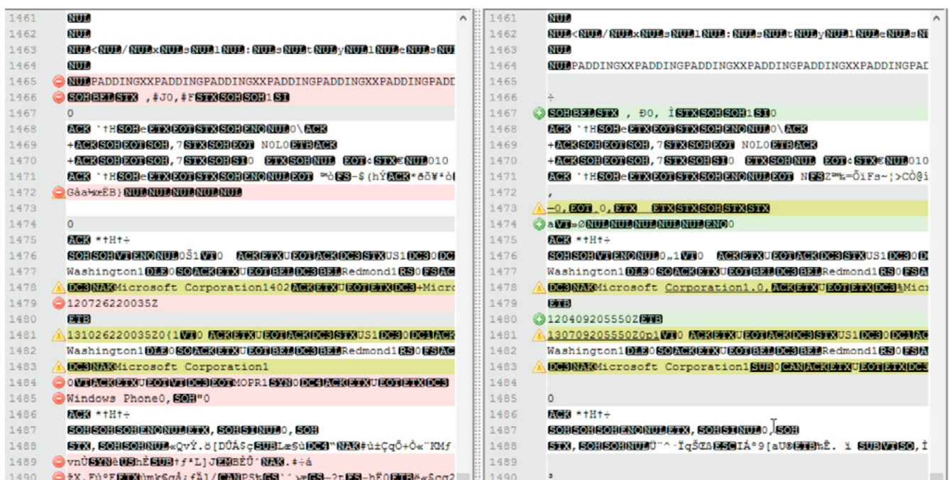
Figure 1. Comparison of Windows Phone 8 and Windows RT boot loaders
