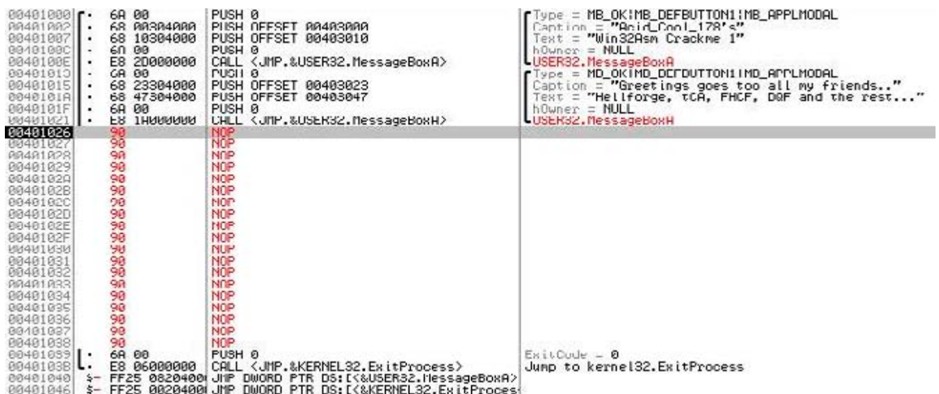
Figure 12. Replaced PUSHes and CALL
