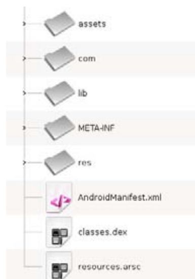
Figure 1. Typical Structure of an APK File
