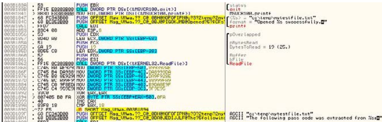
Figure 10. Xor Encryption in Assembler
