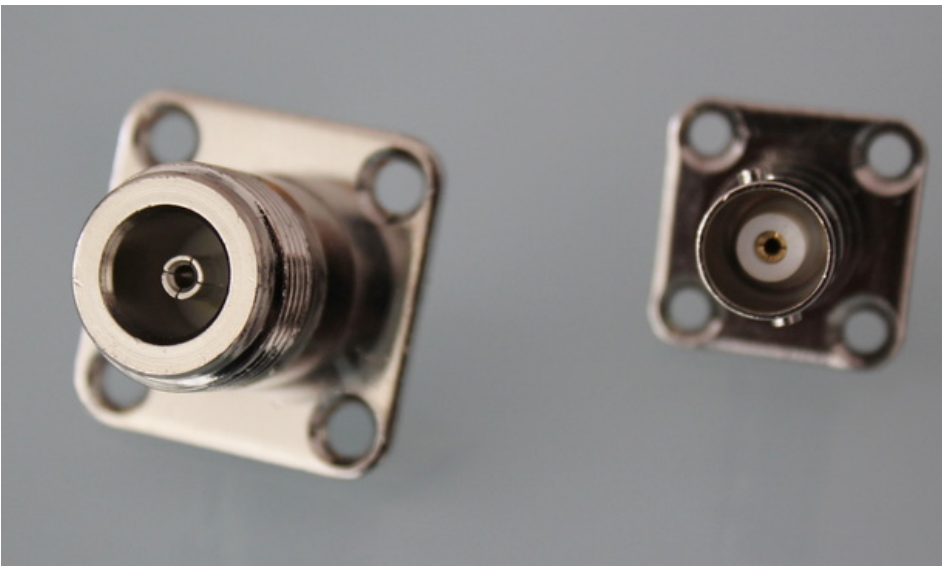
Figure 8. A N-type female chassis-mount connector on the left and its BNC equivalent on the right
