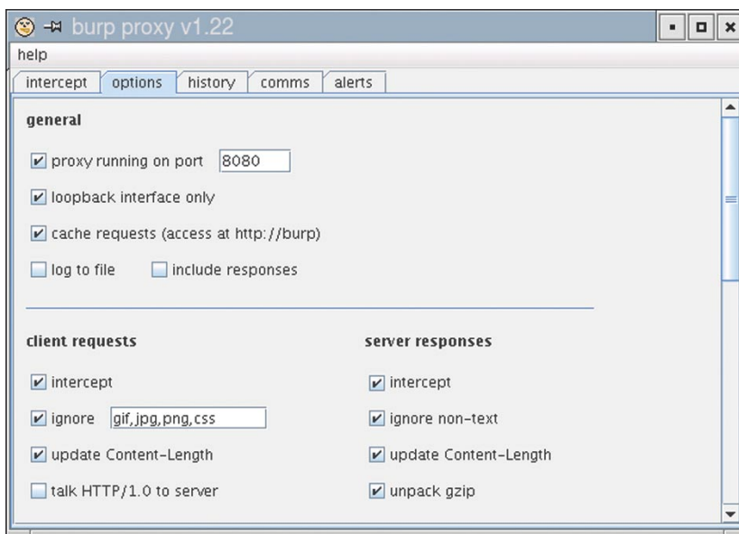
Figure 4. Using burpproxy , in order: launching and configuring burpproxy , configuring Firefox, burpproxy displaying an intercepted request and waiting for us to allow passing it on
