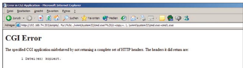
Figure 4. Confirmation after creating a copy of the command shell and the new shell cmd1.exe
