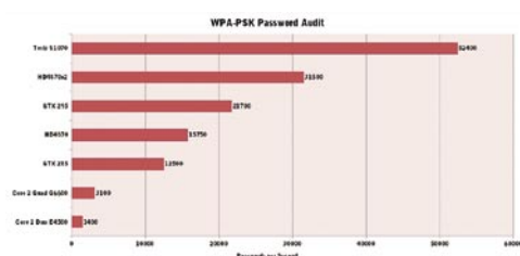
Figure 1. Provided WPA/WPA2 security is used EWSA can find an 8-character password 7 times faster on one GTX 295, compared to Core 2 Quad Q6600
