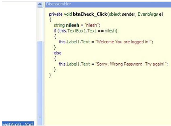
Figure 12. Code for checking password
