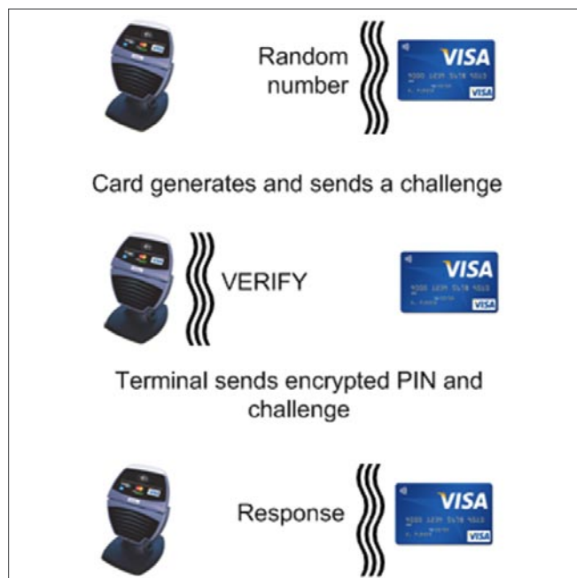
Figure 9. PIN verification protocol
