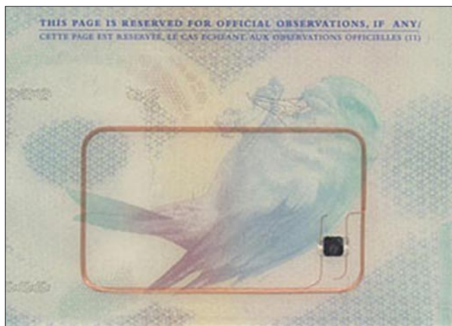
Figure 1. Example: UK Biometric Passport with computer chip
