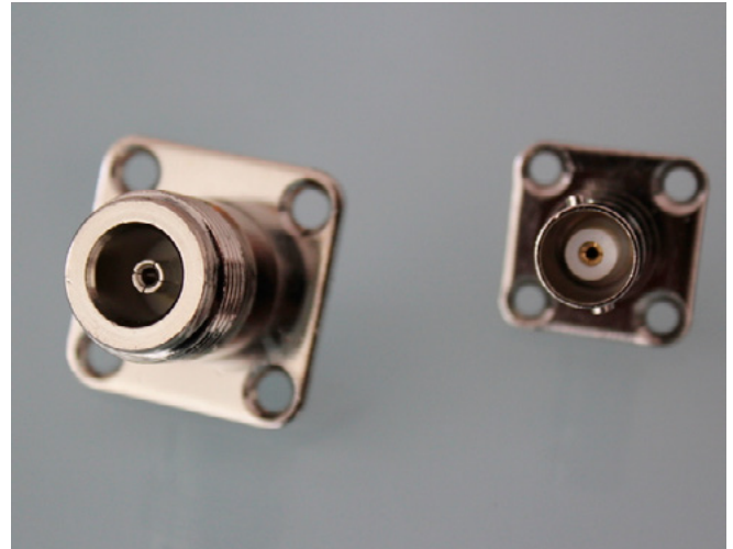
Figure 8. A N-type female chassis-mount connector on the left and its BNC equivalent on the right
