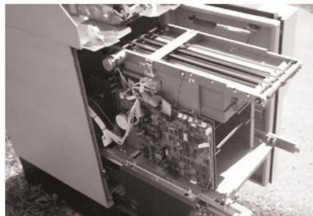
Fig. 4: Rails extended, electronics and cash handler visible
