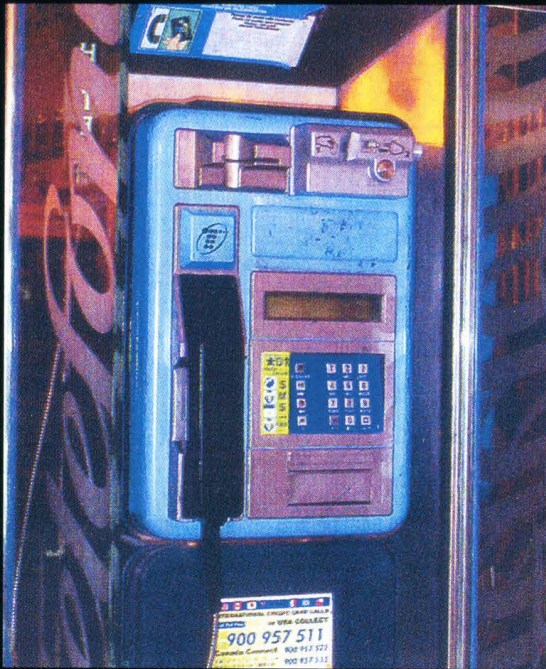
Alicante, Spain. A standard phone throughout the country. It takes credit cards and coins. In addition this phone has SMS and fax capabilities.
