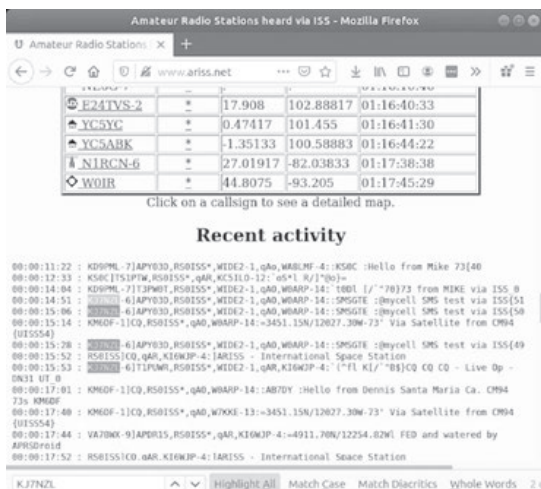
A list of APRS messages retransmitted by the ISS. The highlighted ones are sent by the author.
