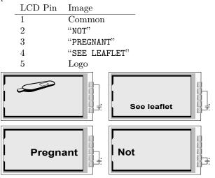
Pin 1 is the rightmost pin if you're looking at the LCD face and the pins are at the top of the package, opposite the reference designator. Make sure to not just short pins—you actually have to lift and move any pins you might be interested in swapping around. Cut a wire here, tack in a jumper there. Mix and match, and get ready to have a ball! Dance a jig! I mean, shoot, a fella could have a pretty good weekend in Vegas with all that.
