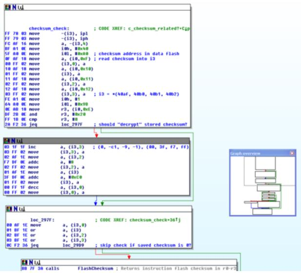
Figure 22: Firmware checksum verification function for version 1.10.
