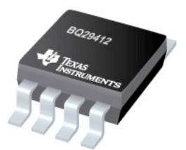
The chip in Figure 7 marked 29412 is a Texas Instruments bq29412 overvoltage protection IC for 2, 3, or 4-cell LiOn battery packs. The bq29412 has a fixed overvoltage protection threshold of 4.45V. If one of the cell's voltages exceeds this threshold for more than a programmable amount of time, an external fuse is blown to prevent further charge.
