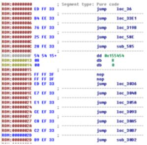
Figure 18: reset and interrupt handlers for the firmware
