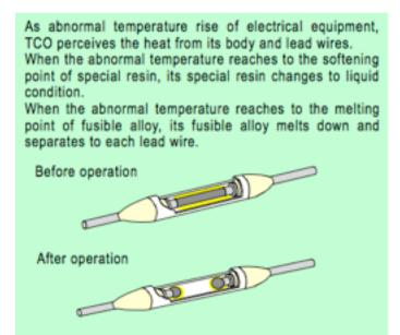
Each cell has a Matsushita MU092X thermal cutoff. If the temperature rises too high, it will permanently cutoff the connection to the cell.
