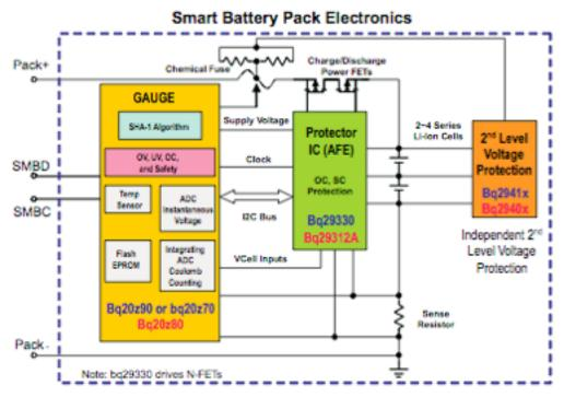
Figure 9: Smart battery electronics
