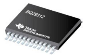
The 29312 chip is a Texas Instruments bq29312 battery protection analog front end (AFE). The bq29312 provides safety protection for overcharge, overload, short-circuit, overvoltage, and undervoltage conditions in conjunction with the battery management host.
