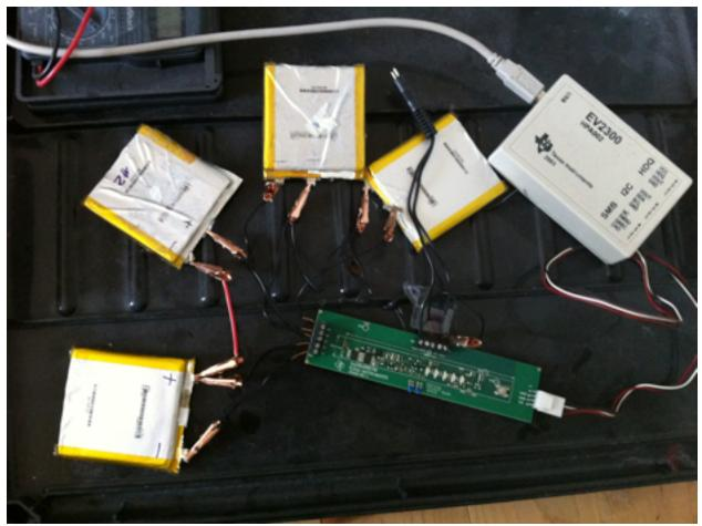
Figure 15: The bq20z80 test rig
