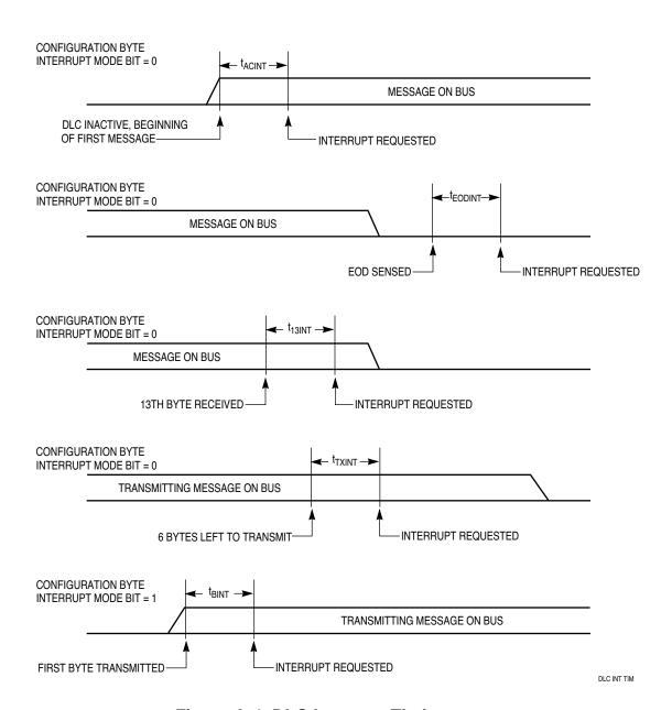
Figure A-4 DLC Interrupt Timing
