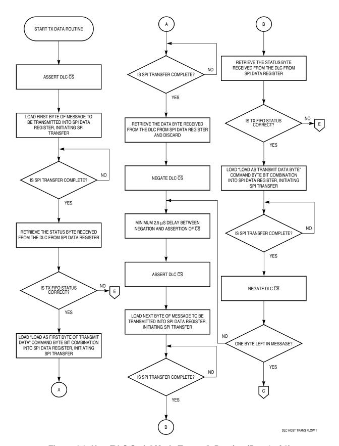
Figure 4-9 Host/DLC Serial Mode Transmit Routine (Part 1 of 2)
