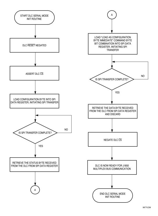
Figure 4-8 Host/DLC Serial Mode Initialization Routine
