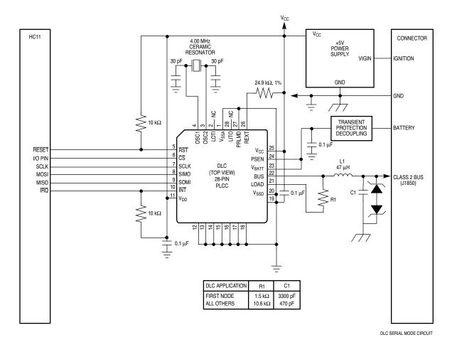
Figure 2-3 DLC Serial Mode Circuit
