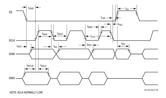
Figure A-2 SPI Timing — Active High SCLK
