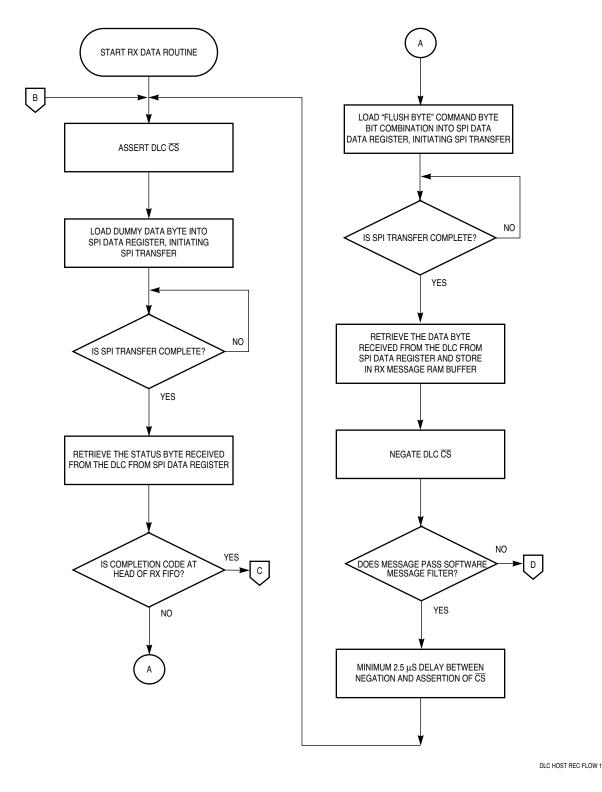
Figure 4-11 Host/DLC Serial Mode Receive Routine (Part 1 of 2)
