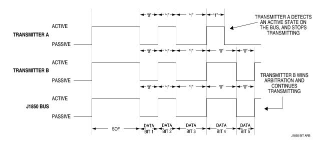
Figure 3-6 J1850 VPW Bitwise Arbitration
