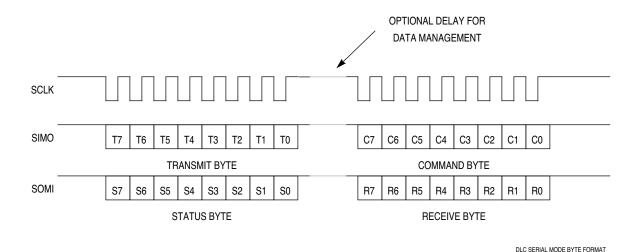
Figure 4-5 DLC Serial Mode Byte Format
