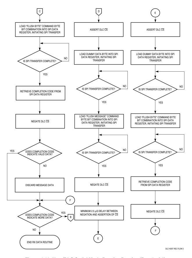
Figure 4-12 Host/DLC Serial Mode Receive Routine (Part 2 of 2)
