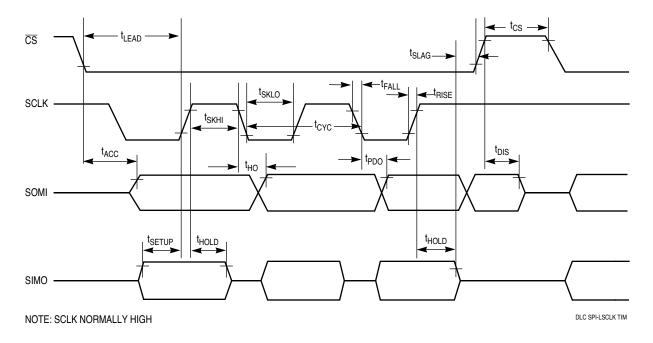
Figure A-3 SPI Timing — Active Low SCLK
