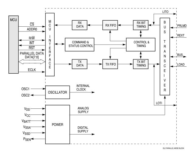
Figure 1-1 MC68HC58 DLC Parallel Mode Block Diagram
