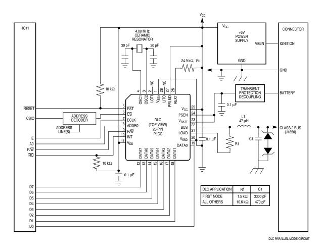
Figure 2-2 DLC Parallel Mode Circuit
