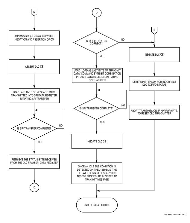
Figure 4-10 Host/DLC Serial Mode Transmit Routine (Part 2 of 2)
