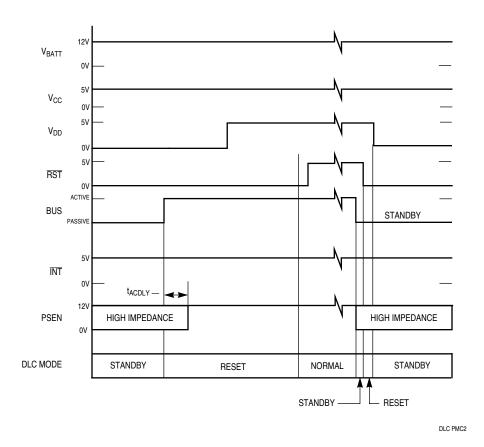
Figure 2-5 Method 2 — Switching V<sub>DD</sub> with PSEN
