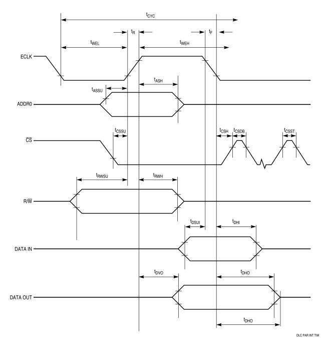
Figure A-1 Parallel Interface Timing
