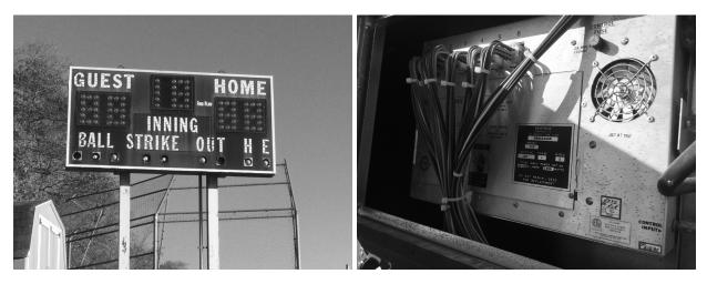
Figure 2: FairPlay 710 scoreboard and internal processor box.
