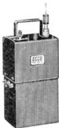
ECCO 10 METER TRANS-RECEIVER Designed for spot frequency use for emergency, CD, and net operation. Completely self-contained including batteries. Transmitter uses 20 meter crystals. Fixed frequency receiver has regenerative circuit. Base loaded 36' antenna. Carbon mike input. 1/2 watt input to final. With 5 tubes. Less mike, headphones, crystal, and batteries.
