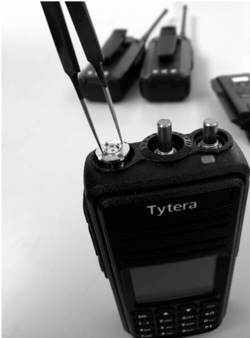
Figure 10.19: Removing the Antenna Rings
