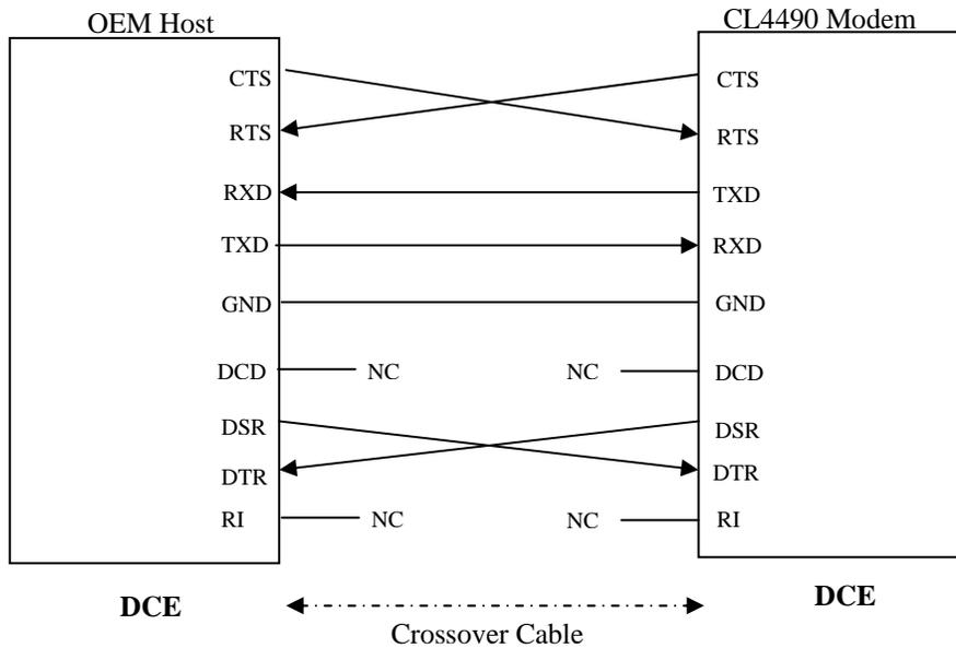
**Note:** The Straight Through Cable provided with the CL4490 has female connectors on both ends and the Crossover cable has a male connector at one end and a female connector at the other end. Please use a male-to-male adapter or female-to-female adapter wherever required. Using a null modem adapter with a Crossover cable is equivalent to using a Straight Through cable.
