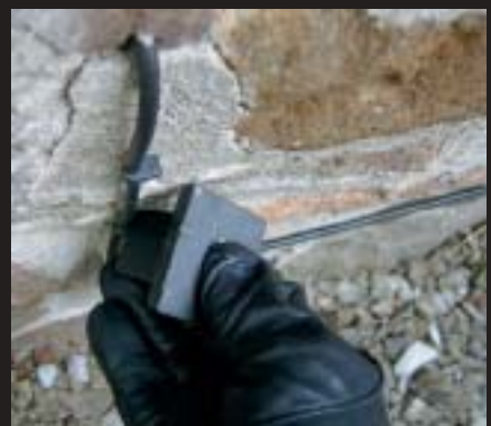
A land-line bug being attached to a phone line
