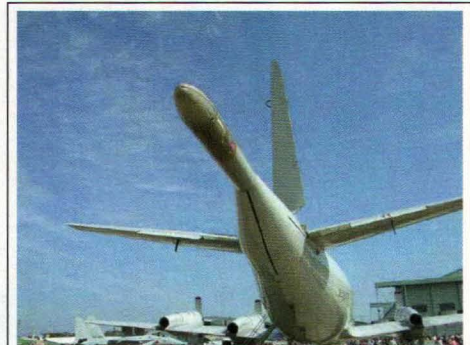
A Lockheed P-3C carrying a magnetic anomaly detector boom - used to find and track submarines
