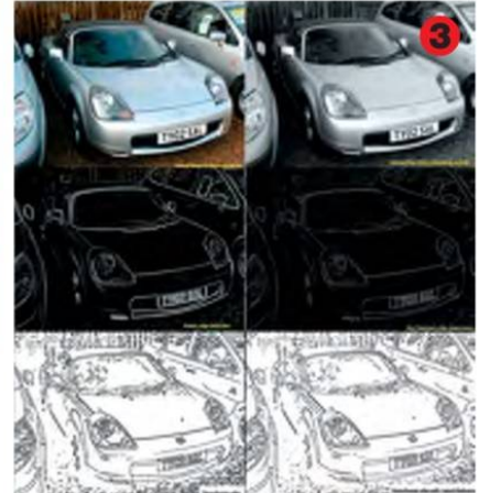
1. An ANPR system atop Brooklyn Bridge in New York. 2. A mobile ANPR system fitted to an Australian police vehicle. 3. How ANPR technology defines a number plate
