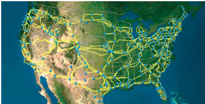
The fibre-optic cable network in the United States is extensive and links all primary populated and defence areas
