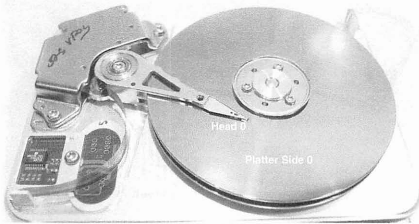
Figure 1–10 Components of a hard disk drive.
