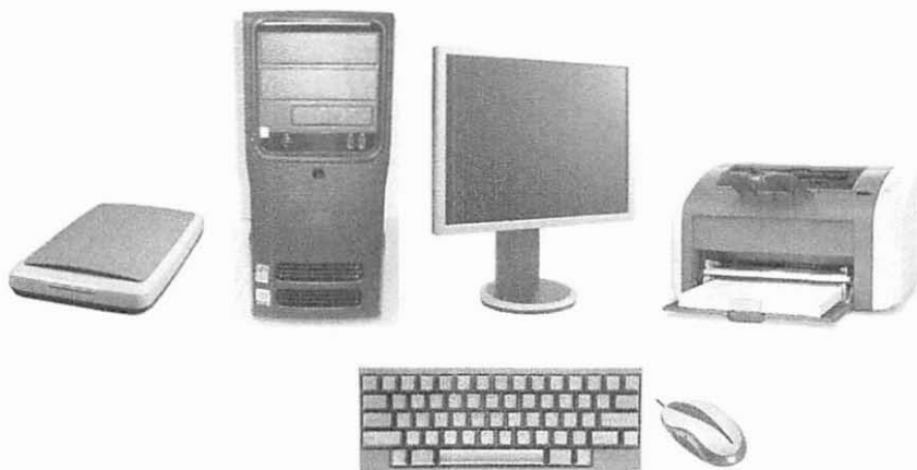
Figure 1-4 Peripheral components that can connect to a computer, including a scanner, a monitor, a printer, a mouse, and a keyboard.
