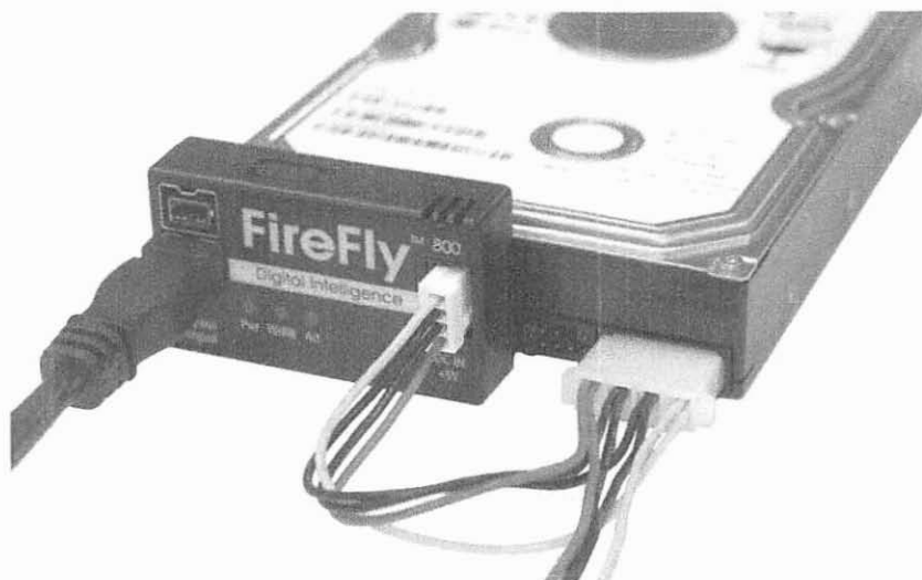
Figure 10-11 A write blocker. Courtesy of Digital Intelligence, Inc. www.digitalintelligence.com
