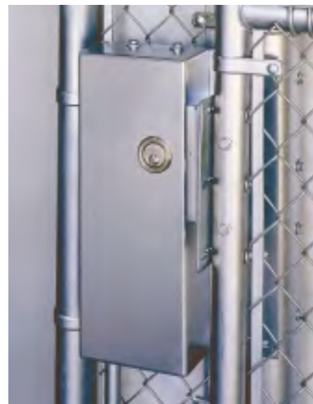
8055 gate lock shown in closed and deadlocked position. When the gate is closed, the locking bolt is completely concealed.
