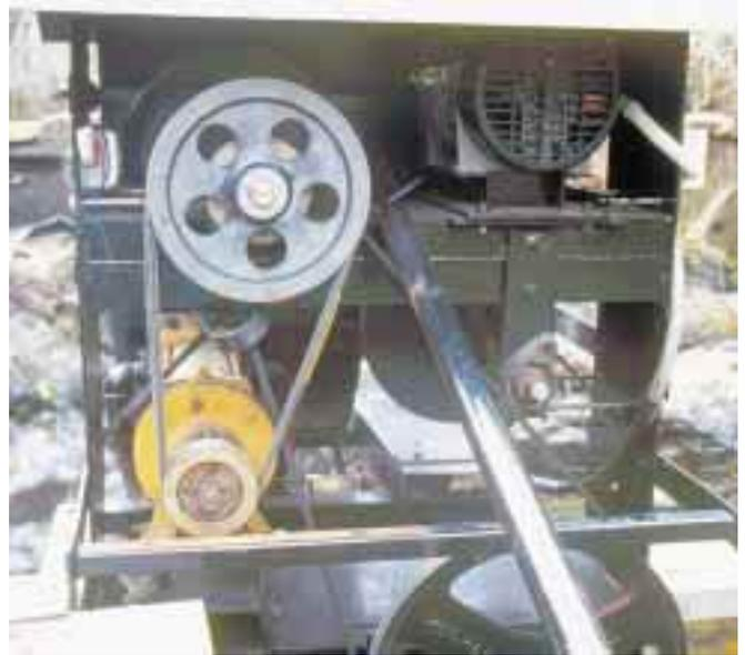
Above: The other side of the Power Tower showing the drive shaft, primary step-up belting, and the pump (in pumping mode).
