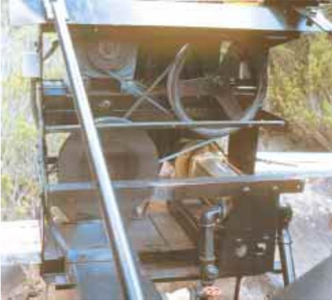
Above: The Power Tower houses the alternator (upper left), the 30 kg flywheel (lower left), and the pump (lower right).
