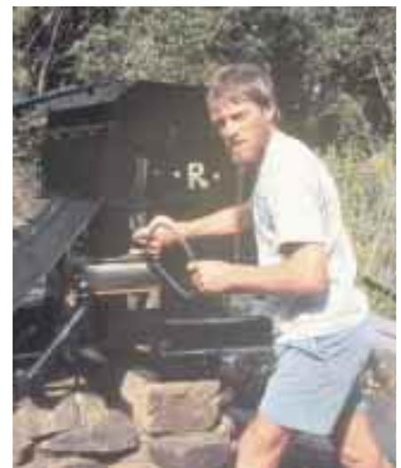
Right: John changes belts to switch the hydro from alternator to pump.
