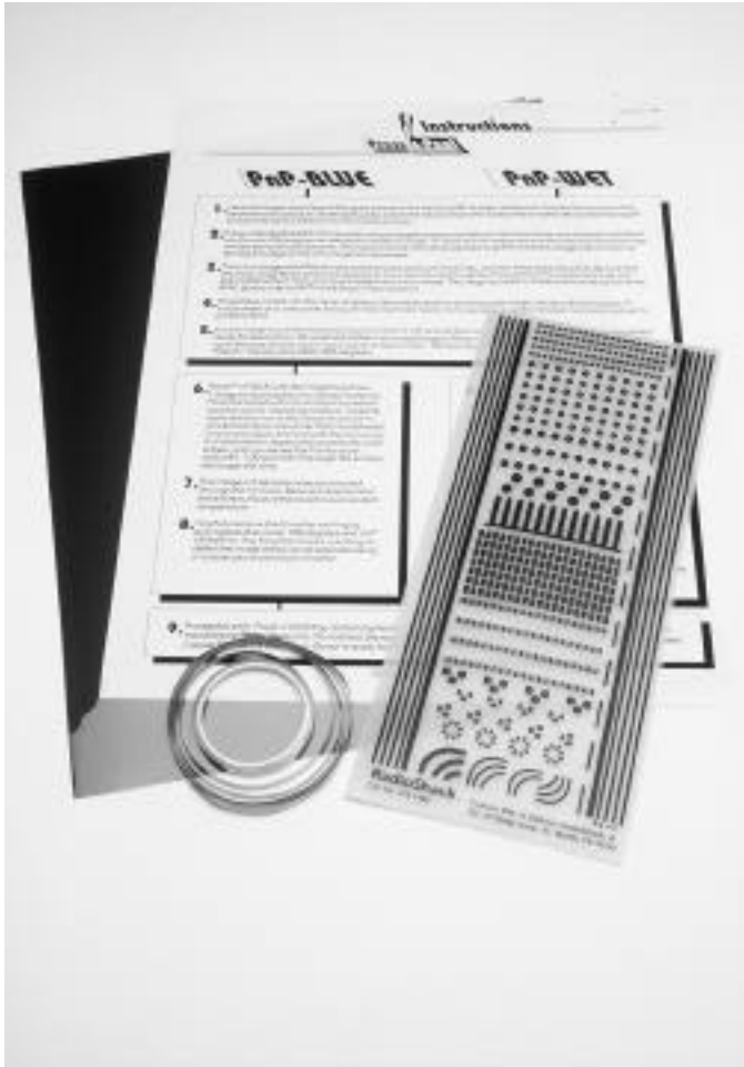
Fig. 13. A variety of techniques are available for prototyping RF boards. PressNPeel (top) can be used to transfer laser printed resist patterns to the board using a steam iron. Rub-on decals (center) can be applied directly to the board. Adhesive backed copper tape (bottom) can be used to create microstrip patterns.
