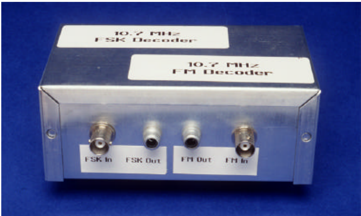
Fig. 10b. Front panel of IF amplifier/decoder box.
