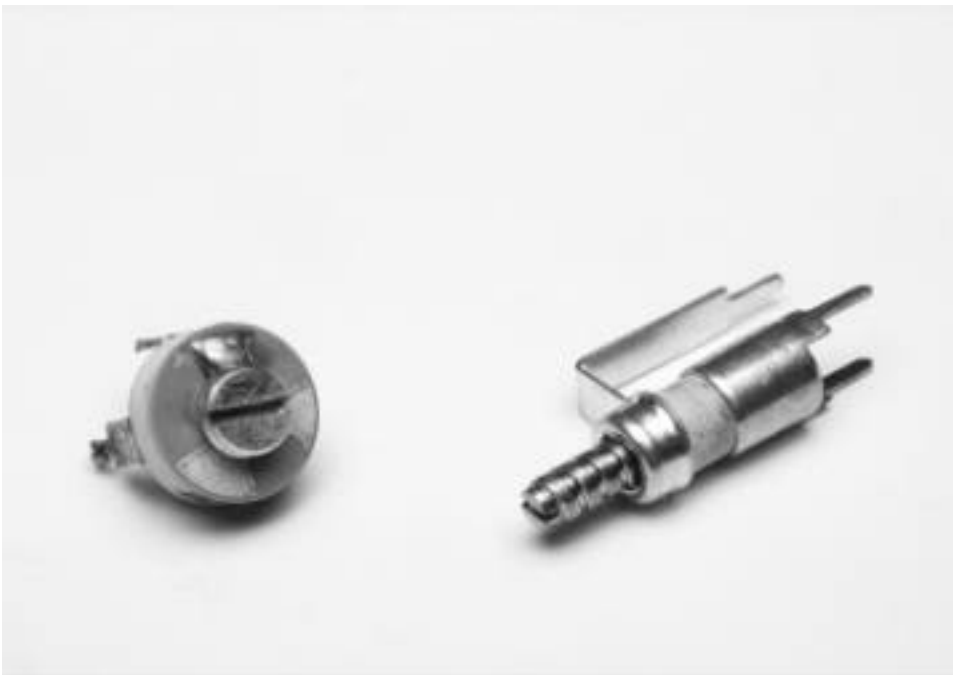
Fig. 4b. Variable capacitors. The ceramic trimmer (left) is useful to about 200 MHz, while versions of the piston cap (right) are available for use above 1 GHz.
