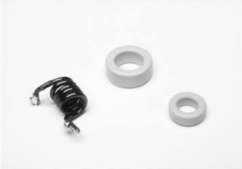
Fig. 3a. A variety of toroidal cores (right) are available for winding inductors at frequencies from a few MHz to about 200 MHz. Air core inductors (left) can be used at VHF and UHF frequencies. There are also chip inductors that are available in small values of inductance.
