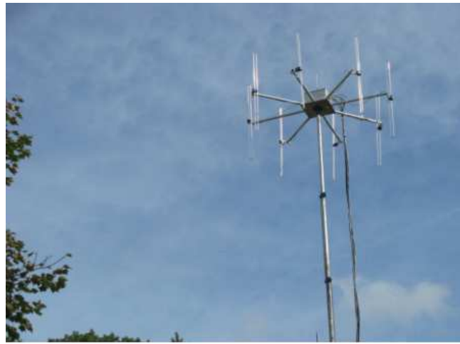
Figure 9: PaRaDe antenna (courtesy of Technical University of Warsaw).
