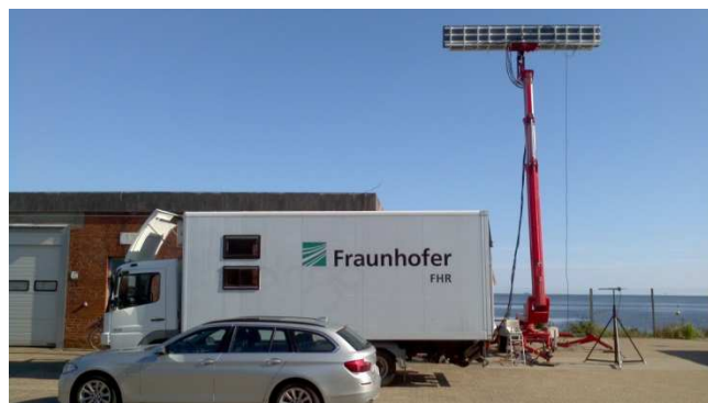
Figure 10: LORA11 DVB-T PCL-System of FHR and FFI with linear array antenna.
