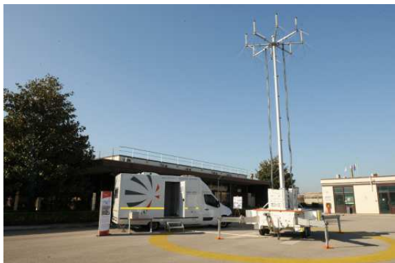
Figure 6: AULOS PCL-system (courtesy of Selex-ES).
