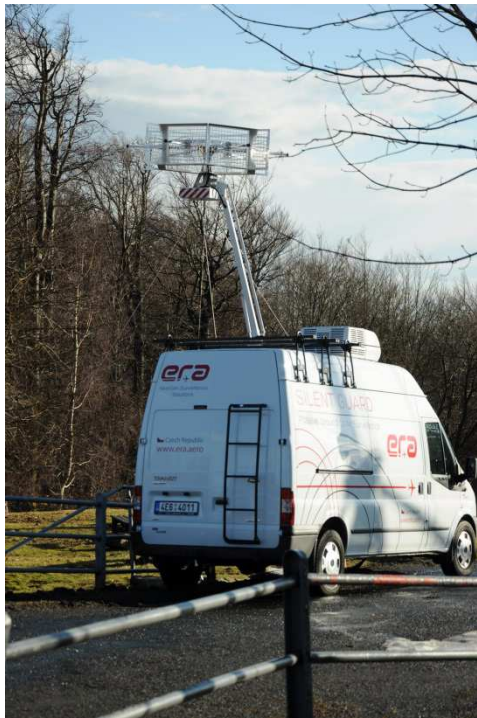
<- Figure 8: ERA 6-element FM-PCL-System.
