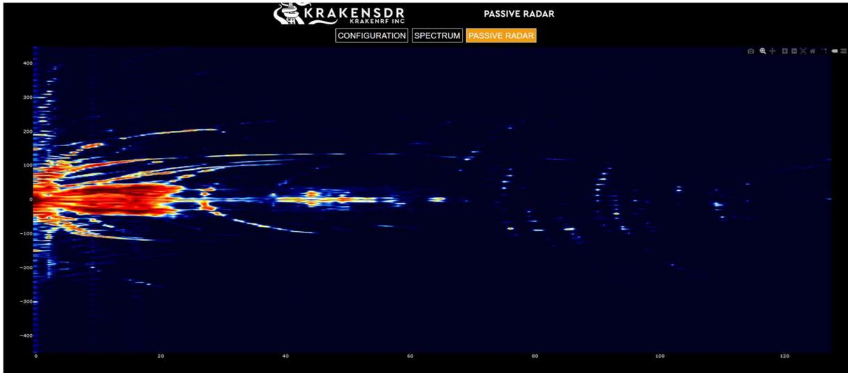
The ellipse segments are traces of aircraft passing in a straight course at various radial speeds and bistatic (= signal path) distances. With my current setup of DAB radio transmitter position and power, its radiation characteristics, my antenna, KrakenSDR parameter settings etc. I am able to detect aircraft at up to about 100 km bistatic distance or 50 km effective range.
