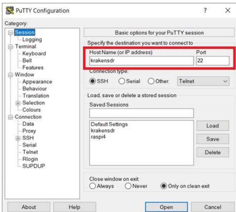
The Pi's SSH server to which Putty on your PC or mobile connects terminates Putty sessions after a timeout. If you want to keep your Putty connection open for a long time without console input from your side, you will have to either cancel the timeout on the Pi's side or activate a "keepalive" function in Putty. You will find instructions for this here:
