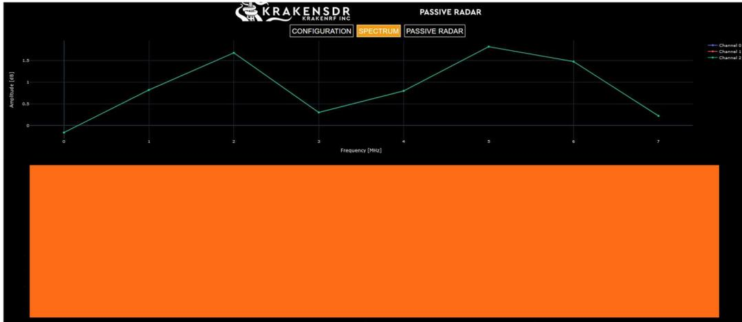
for a few seconds you should then see the CH0 and CH1 spectrums at around -40 dB and left/right centred above a waterfall diagram:
