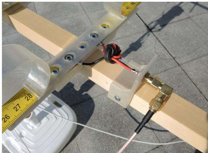
I am talking about the first variant here. Take a small ferrite toroid and wind the thin two-wire line between the dipole and the coaxial cable a few turns (I use four) in parallel (!) onto the ferrite.
