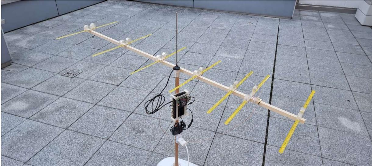
This is my current KrakenSDR passive radar setup: The KrakenSDR and a well-cooled Pi 4 mounted inside my 3D-printed frame and attached to a wooden 25 mm pole, together with a 33 W USB power supply. On top of the pole a  $\lambda/4$  rod antenna connected to KrakenSDR's channel 0. Attached to the pole a self-made 227.4 MHz Yagi connected to KrakenSDR's channel 1.
