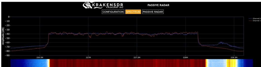
If you observe the big orange square for an extended period of time (tens of seconds), then you either have not started processing or the KrakenSDR may be receiving an insufficient signal level on at least one of CH0 or CH1, i.e. at least one of the antennas may not be connected or the gain of at least one of CH0 or CH 1 may be grossly insufficient, or the transmitter may be off.
