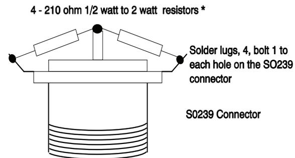
Use a mating connector, a dual male PL259 (Radio Shack #278-192 or equivalent) to connect this directly to the transmitter output SO239
