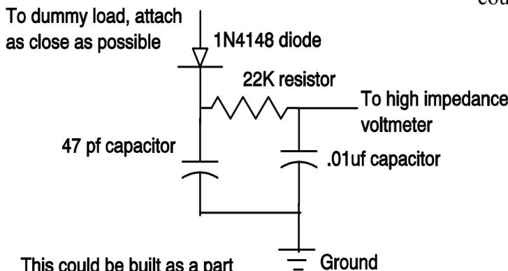
This could be built as a part of the dummy load shown in a previous diagram, keep lead lengths as short as possible
