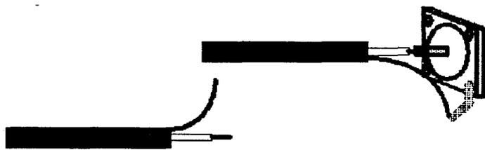
Open up the braid near the insulation by pushing it back to form a small opening through which the inner conductor will be pulled
