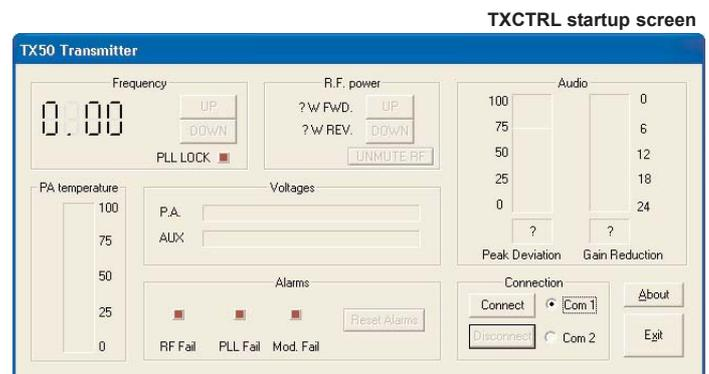
Connect a serial cable between the RS232 board that plugs into the i-o D-type on the rear of the transmitter and one of your computers COM ports. If you are using a codec or other device then you may be able to connect that device in line to act as part of the serial link.
