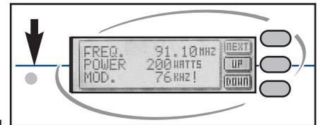
The maximum power set is positioned to the lower left of the LCD screen on some models, other models may not have the hole in the front panel and you will need to remove the lid of the transmitter to access the adjustment which will be in the same position but on the other side of the PCB. You will need a small 'tweaker style' flathead screwdriver to adjust the pot. This control is quite delicate so try to not be too heavy handed in it's adjustment.
