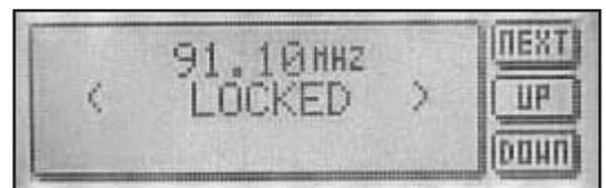
*The LCD readout will only display frequencies in 100Khz steps. Any frequency offsets derived from the internal 12.5KHz offset switch will not show on the LCD. Consult a frequency counter if using offsets.*
