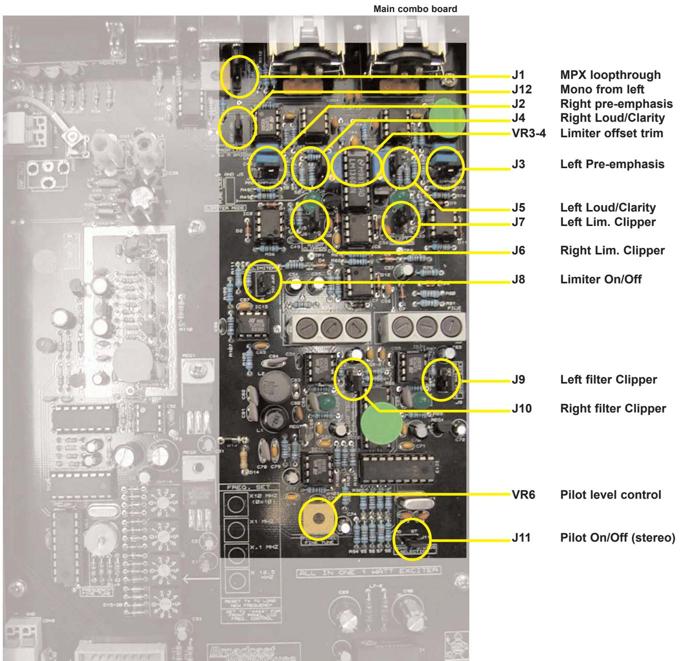
There are altogether twelve jumpers on the board which can be set - at the time of installation - to establish the way the board operates.
