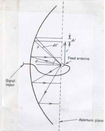
Efficiency factor has an ideal value when only field non-uniformity in the aperture plane is taken into account of  $K = 55\%$ . Empirically,  $K \sim 40\%$
