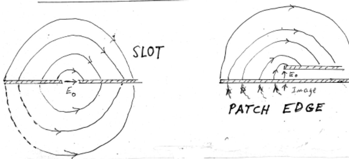
*Radiation from patch edge is like radiation from a slot, but it is only into a half space. However, with image on ground plane, there are equivalently 2 antennas radiating into the half space.*
