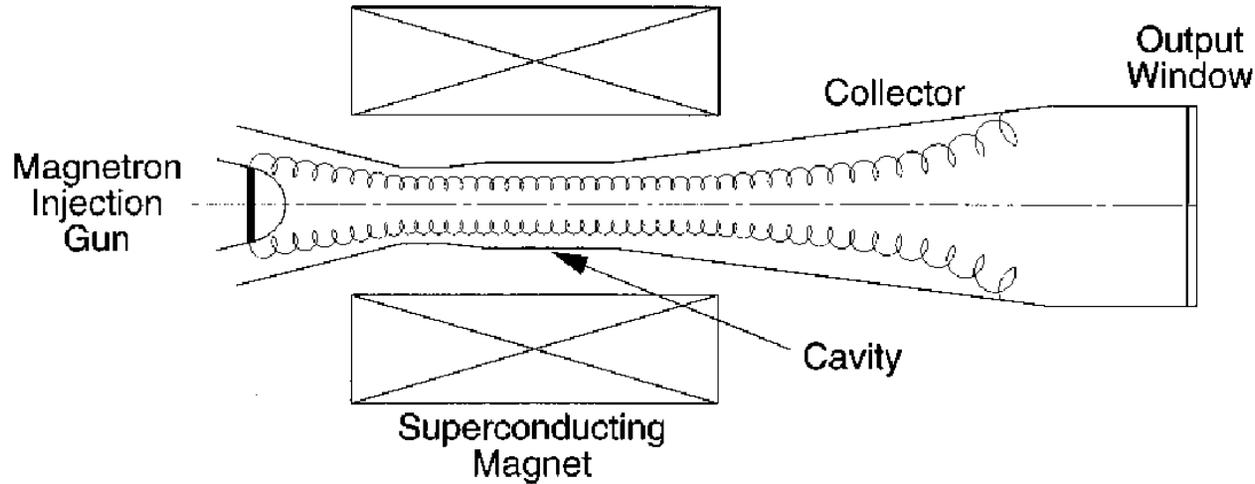
**Gyrotron is a specific configuration of CRM comprising a magnetron-type electron gun and an open microwave structure for producing high-power millimeter-wave radiation**
