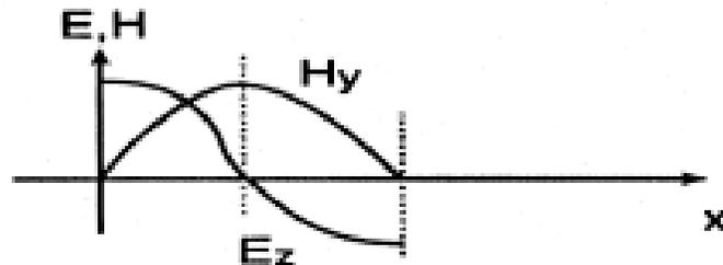
$E_z$  field along edges at  $X=0$  and  $X=a$  looks like magnetic equivalent of dipole antennas which are in-phase.
