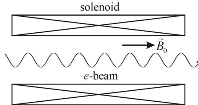
In the cyclotron resonance condition  $\omega - k_z v_z = s\Omega$
