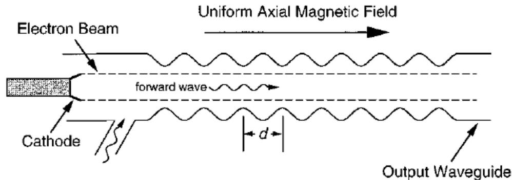
When the electron velocity slightly exceeds the wave phase velocity, the wave withdraws a part of the beam energy. This leads to amplification of the wave.
