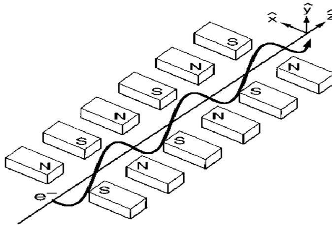
**Example: electron motion in a wiggler, which is a periodic set of magnets**
