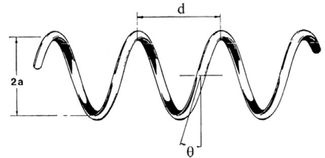
Phase velocity of the wave along the axis  $v_{ph} = c \sin \theta$
