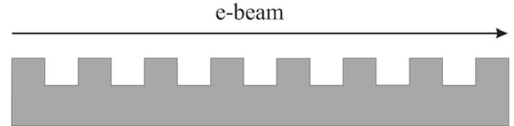
When there is a periodic structure (with a period  $d$ ) confining EM waves, the fields of these waves can be treated as superposition of space harmonics of the waves (Floquet theorem)
