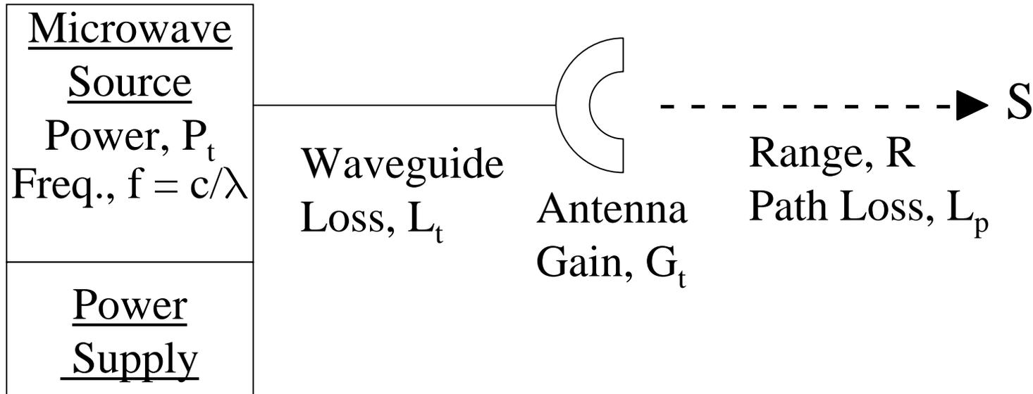
Effective Isotropic Radiated Power,  $EIRP = P_t G_t / L_t$
