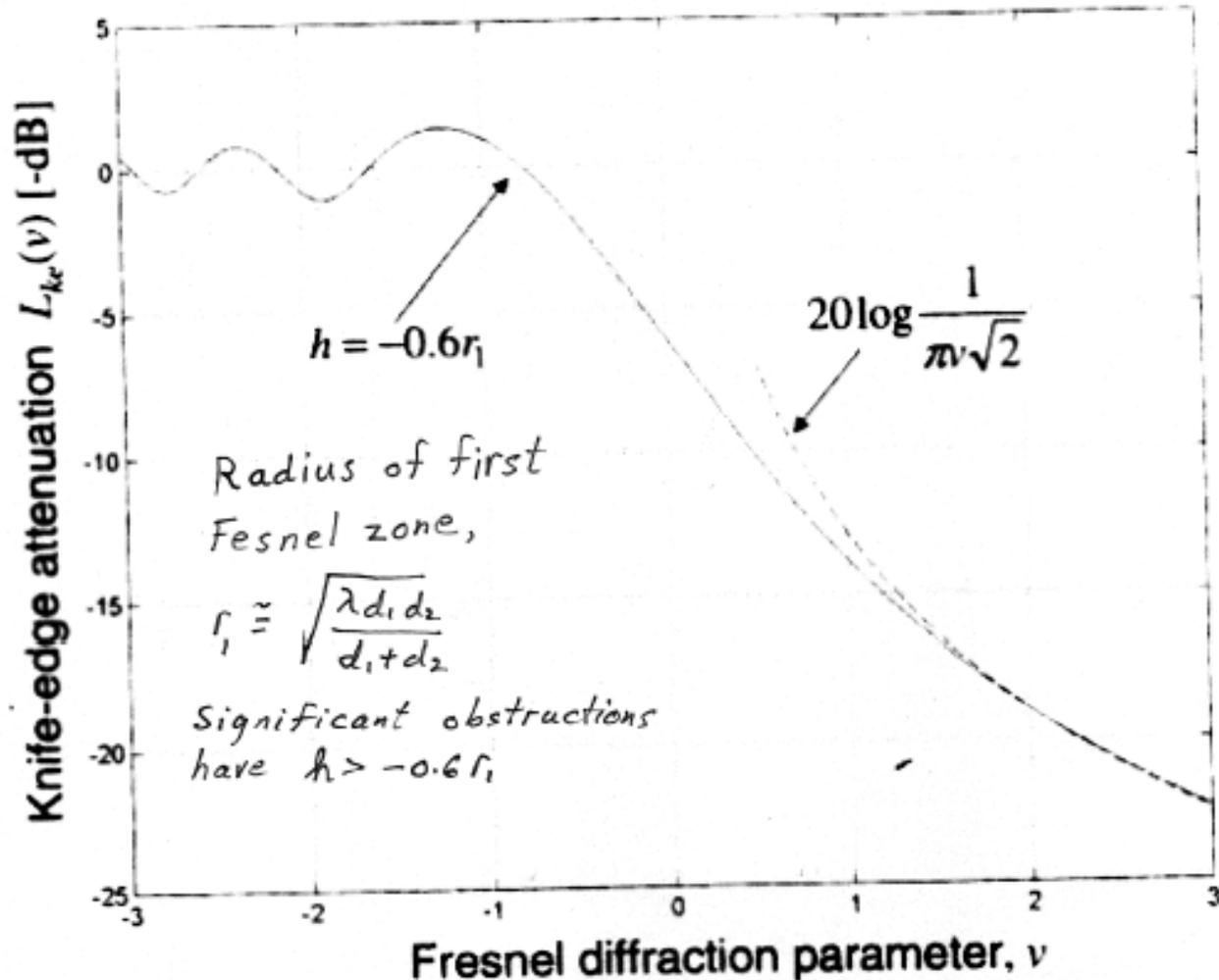
3.15: Knife-edge diffraction attenuation: (—) exact (---) large  $\nu$  approximation
