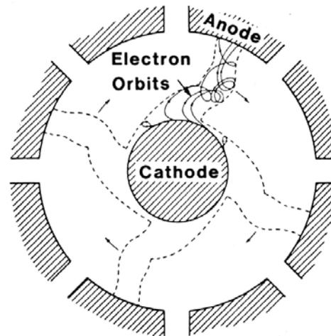
**Electron spokes rotate synchronously with the EM wave rotating azimuthally**
