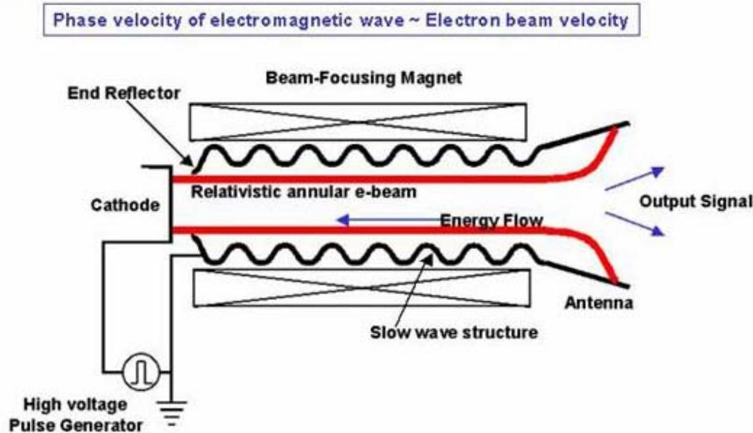
In BWOs, there is the synchronism between electrons and the positive phase velocity of the wave, but the group velocity is negative that means that the EM energy propagates towards the cathode. (Internal feedback loop) Then, this wave is reflected from the cutoff cross-section and moves towards the output waveguide without interaction with the beam.
