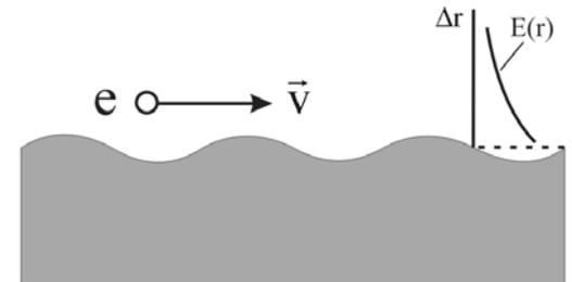
As the beam voltage increases, the electron velocity approaches the speed of light. Correspondingly, the wave can also propagate with the velocity close to speed of light. (Shallow slow-wave structures)
