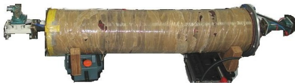
Millimeter-wave stun-gun prototype under construction in the CJS lab
