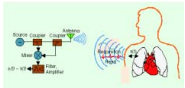
Fig. 1 A single antenna system with single subject. A homodyne radio is used to detect the phase shift proportional to chest displacement due to cardiopulmonary activity.
