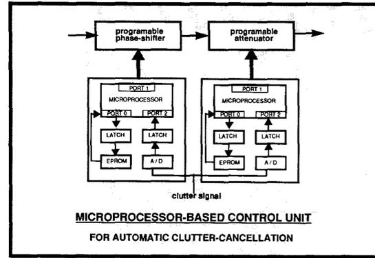
Fig. 3. Circuit diagram of the microprocessor-based control unit for automatic clutter-cancellation.
