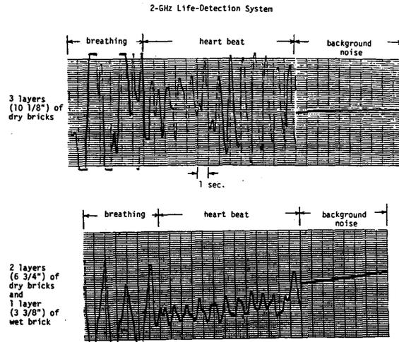
Fig. 9. Heart and breathing signals of a human subject measured through walls of dry and wet bricks with the 2-GHz microwave life-detection system. One layer of wet bricks had a considerable but not severely hampering effect on the penetration of the microwave beam.
