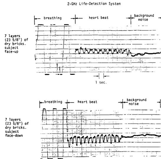
Fig. 7. Heart and breathing signals of a human subject, lying with face-up or face-down position under seven layers of bricks, measured by the 2-GHz microwave life-detection system.
