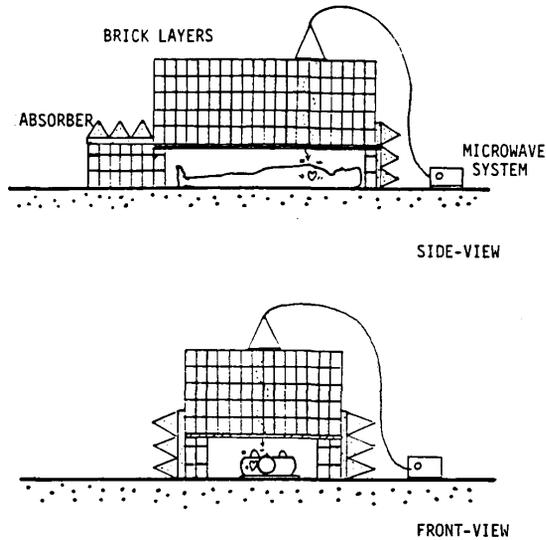
Fig. 4. Experimental step for the measurement of heart and breathing signals of a human subject under layers of bricks using the microwave life-detection system.
