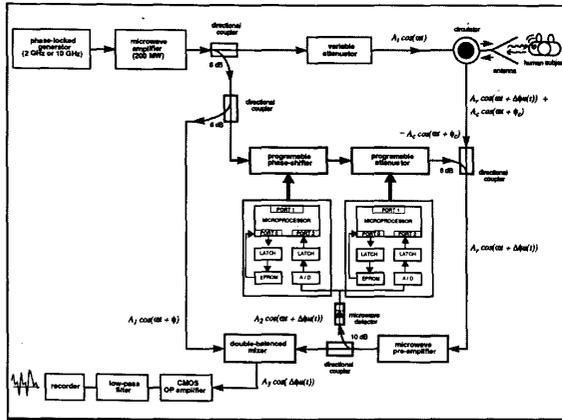
Fig. 2. Block diagram of the microprocessor-controlled microwave life-detection system.
