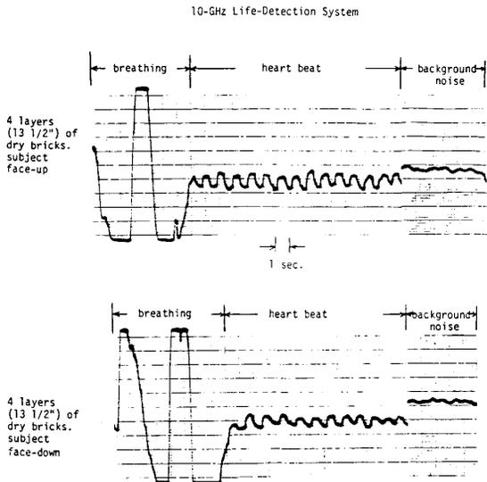
Fig. 5. Heart and breathing signals of a human subject, lying with face-up or face-down position under four layers of bricks, measured by the 10-GHz microwave life-detection system.
