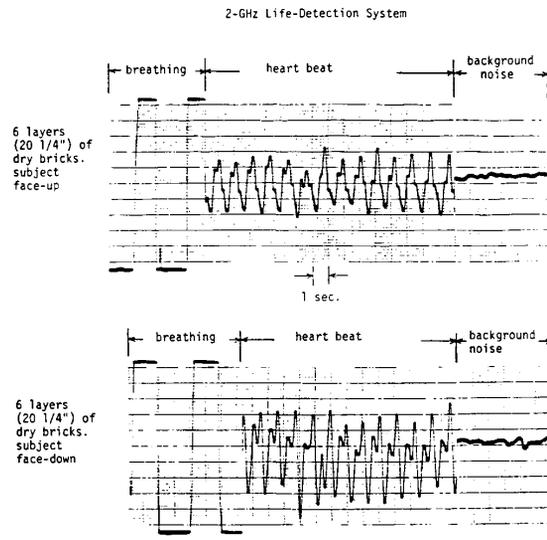
Fig. 6. Heart and breathing signals of a human subject, lying with face-up or face-down position under six layers of bricks, measured by the 2-GHz microwave life-detection system.
