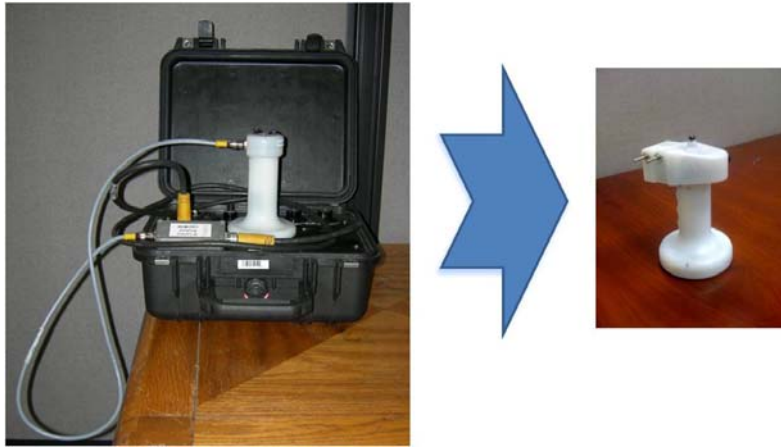
Figure 8. In the Wireless Handheld System, the microwave interferometry instrument electronics and controls have been incorporated into the Probe Assembly, which communicates by Bluetooth with the User Interface Computer. A miniature computer or display device functions as the operator interface.
