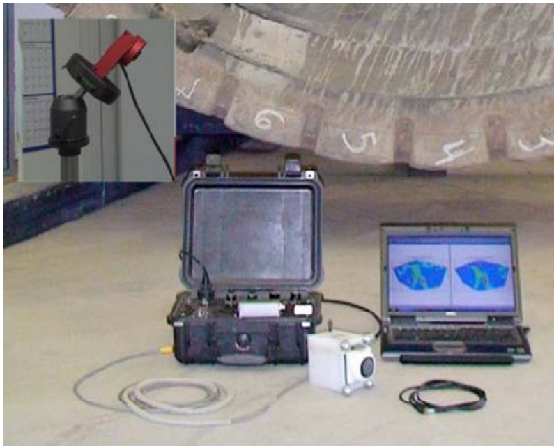
Figure 6. Portable microwave interferometry equipment configured with infrared position tracking
