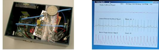
Figure 1. Smart-it with radar (l.), PC client (r.)
