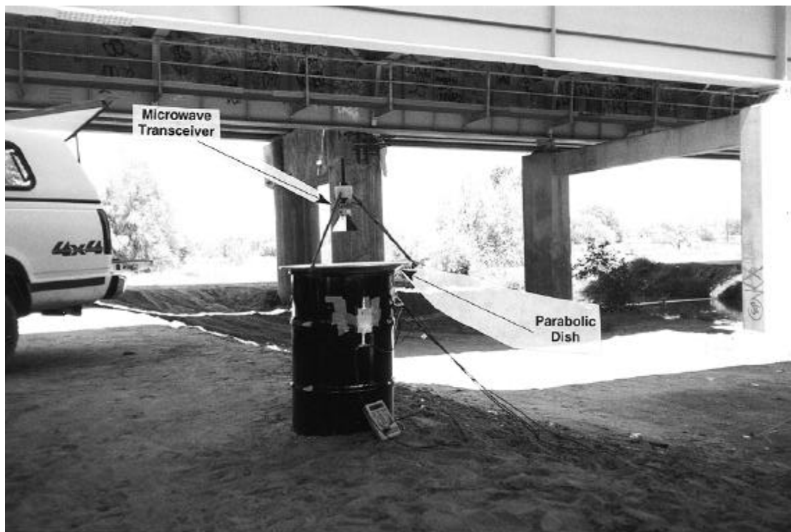
Fig. 2. The microwave interferometer setup in the field to measure the response of a plate girder.
