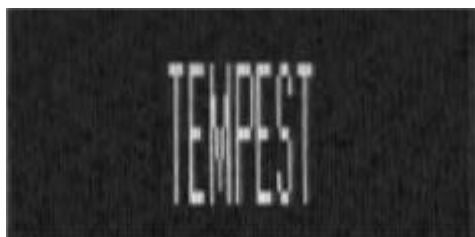
Figure 10. Reconstructed image from the output of the four channel signal enhancer
