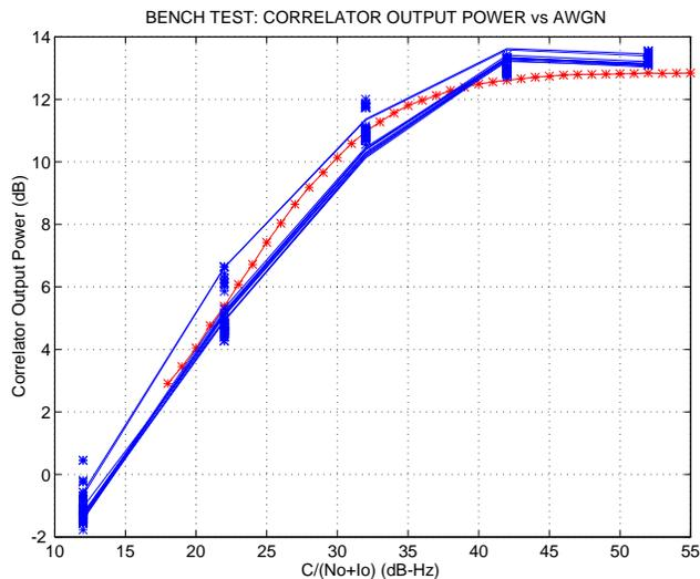
Figure 13: Correlator Output Power vs  $C/N_0$ , AWGN, for Bench Test and Simulation.
