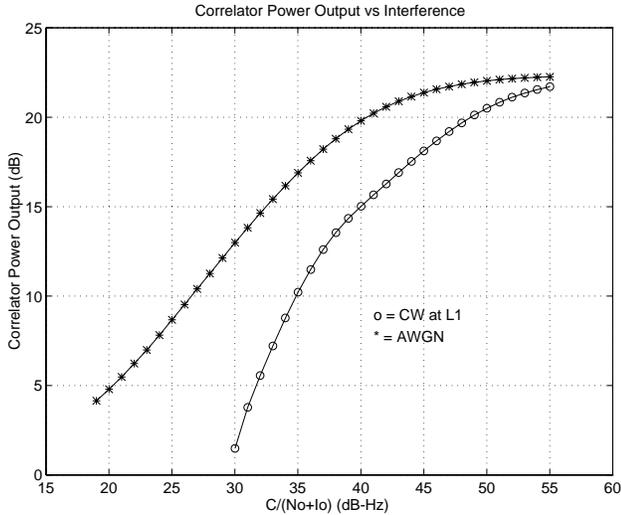
Figure 8: Correlator Output Power vs.  $C/(N_o+I_o)$  for AWGN and CW Interference
