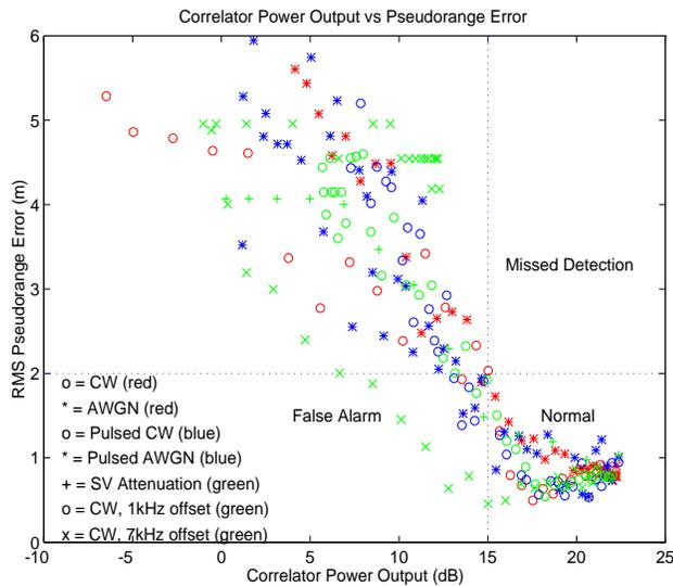
Figure 9: Pseudorange Error vs. Correlator Output Power
