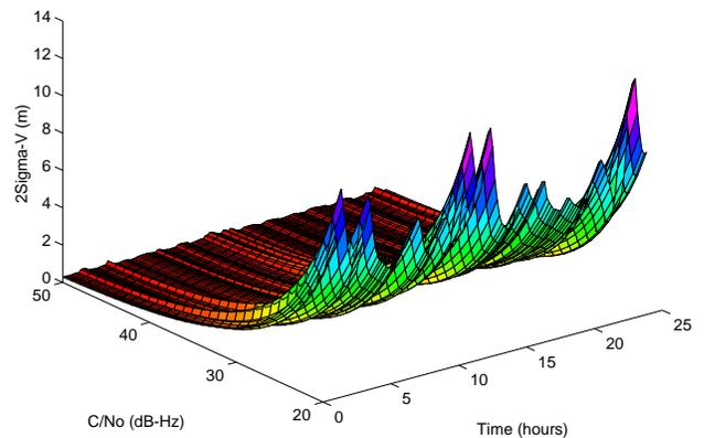
Figure 16:  $2\sigma_v$  vs.  $C_{zenith}/(N_0+I_0)$  over time for DGPS
