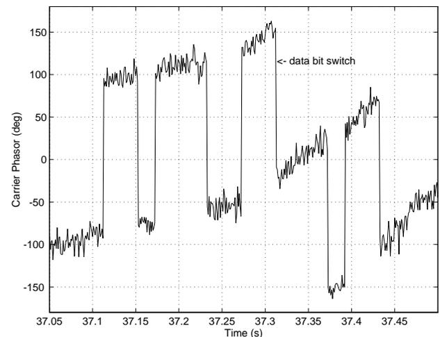
Figure 4: Carrier Phase for a GPS Receiver with a FLL Carrier Tracking Loop
