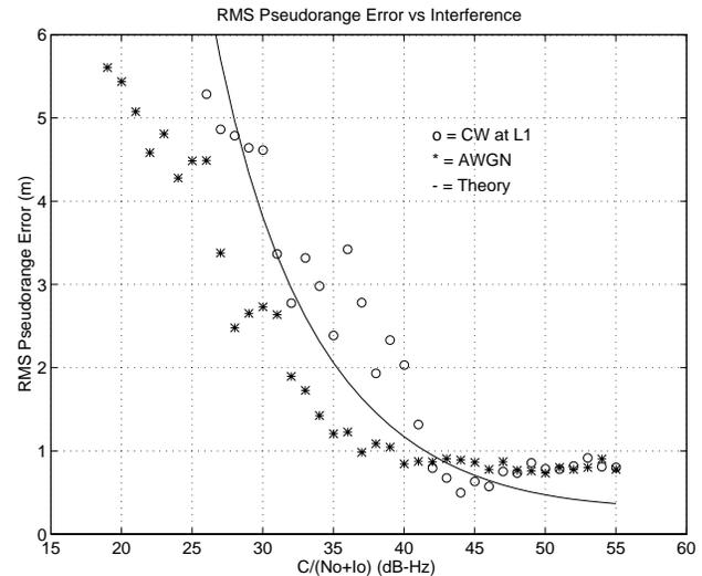
Figure 1: Pseudorange Error vs.  $C/(N_o+I_o)$  for AWGN and CW Interference
