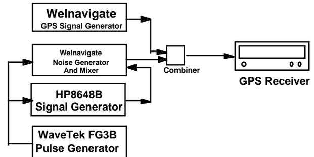
Figure 6: Bench Test Setup
