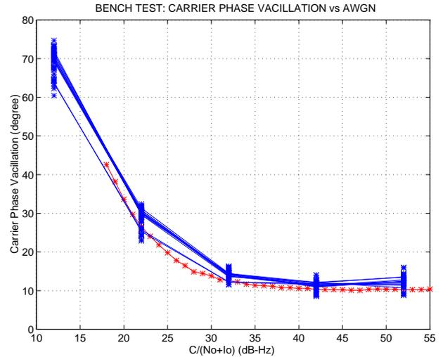
Figure 15: Carrier Phase Vacillation vs  $C/N_0$ , AWGN, for Bench Test and Simulation.
