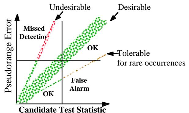
Figure 7: Test statistic characteristics
