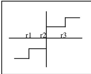
Figure 5: 2-Bit Quantizer Thresholds (AGC gain)
