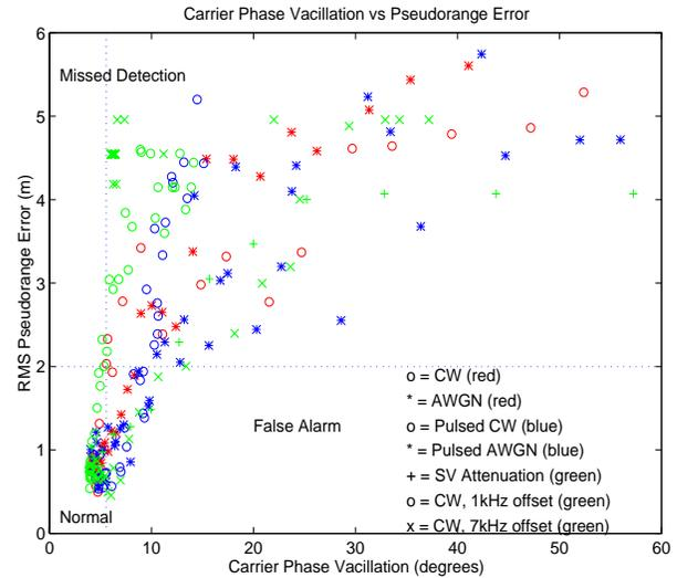
Figure 11: Pseudorange Error vs. Carrier Phase Vacillation.
