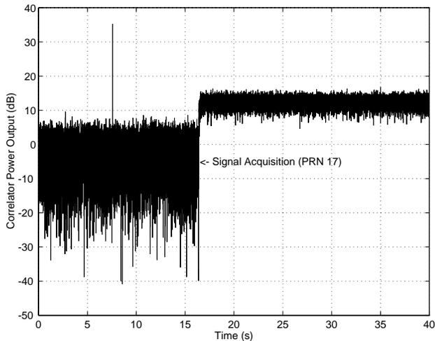
Figure 3: Correlator Output Power for a GPS Receiver
