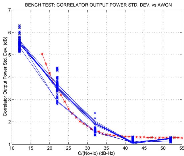
Figure 14: Correlator Output Power Variance vs  $C/N_0$ , AWGN, for Bench Test and Simulation.
