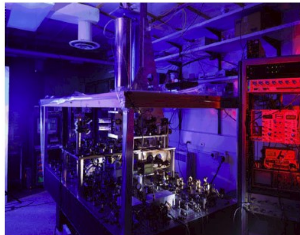
NIST-F1 Cesium Fountain Atomic Clock The Primary Time and Frequency Standard for the United States
