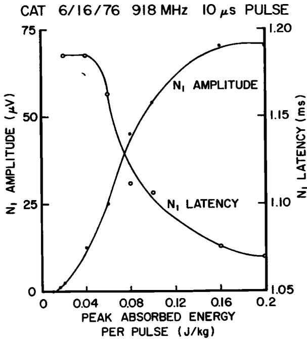
Fig. 6. Amplitude of microwave-induced  $N_1$  and latency of  $N_1$ , as a function of the peak absorbed energy per pulse.
