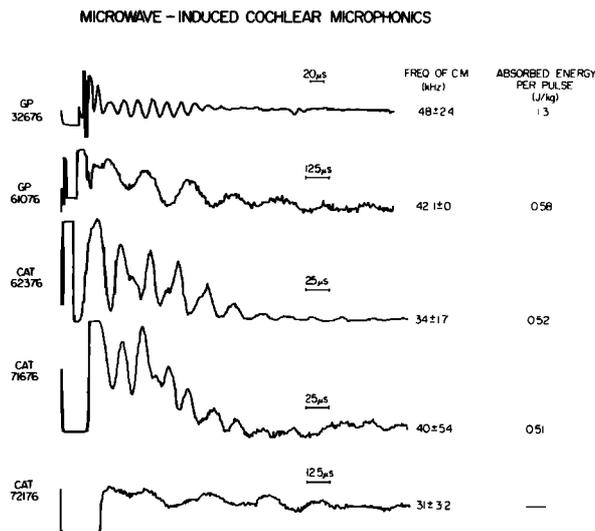
Fig. 1. Microwave-induced cochlear microphonics in guinea pigs and cats. Pulsed microwave: 918 MHz, 10  $\mu$ s width.
