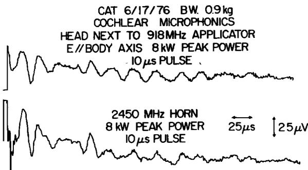
Fig. 3. Comparison of cochlear microphonics induced by pulsed microwaves at  $918$  and  $2450 \text{ MHz}$ .
