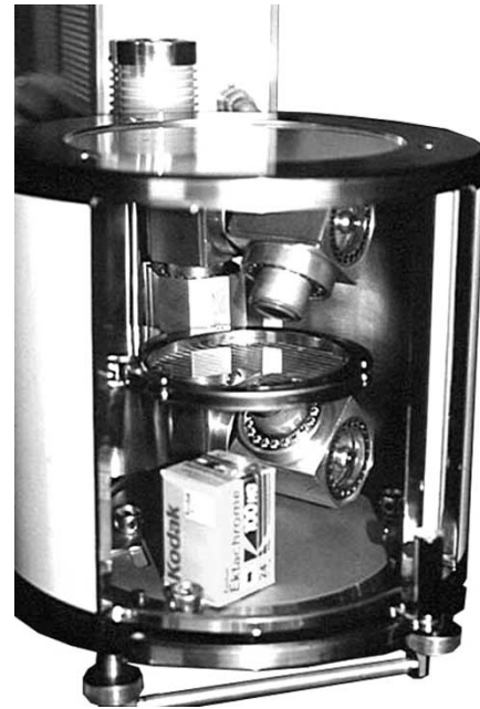
Fig. 15. System of two sealed-off e-beam vacuum diodes of a laboratory technological accelerator, which are placed in a compact protective chamber.
