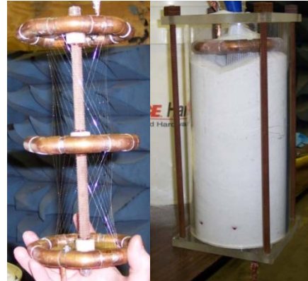
Fig 6. Fuse is shown with wires and field shapers (left). The fuse is packed with fine glass beads (right).
