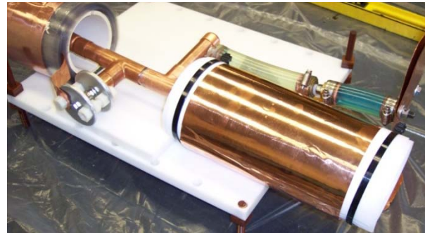
Fig. 8 Full system load with pulse transformer at upper left.
