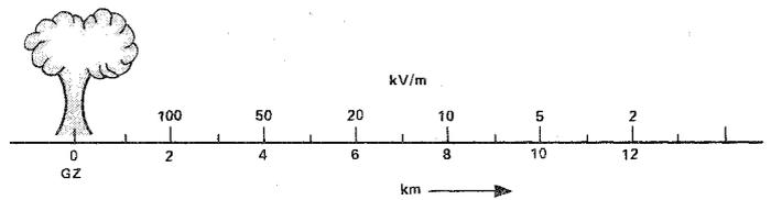
Fig. 2. The field strengths produced by detonating a one Megaton bomb. Remember too that a 20 Megaton warhead is very commonplace today - and to be expected in combat.
