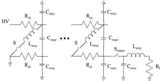
Figure 3. The Wave-Erection Marx Generator.
