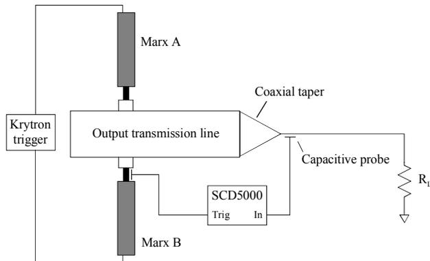
Figure 6. Experimental arrangement.
