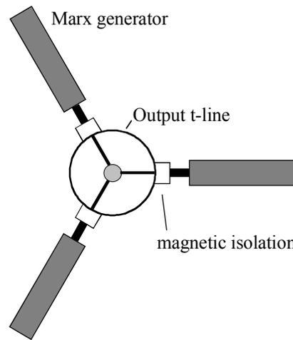
Figure 5. Generator interconnection with output transmission line
