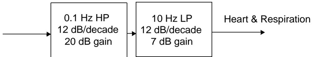
**Figure E.7.** Configuration of SR560 preamplifiers for quadrature measurements.
