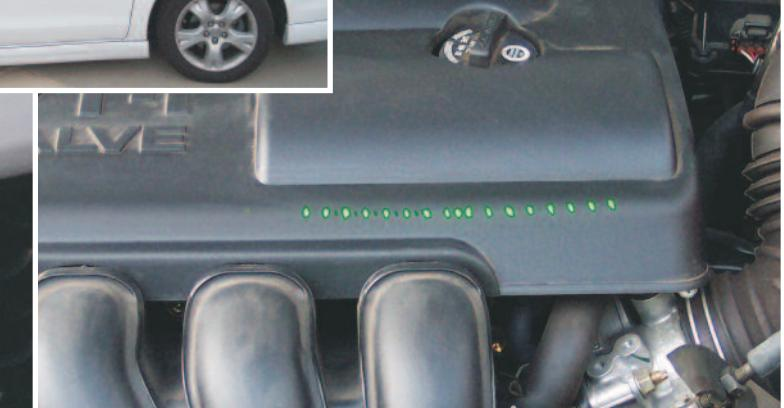
Since all the multiple points are measured at the same time, transient events can be accurately measured. In addition, the relative phase between measurement locations can be used to generate modal vibration patterns in a single shot.
